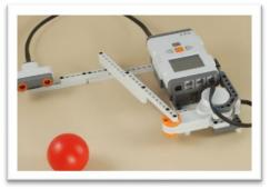
The Baseball Batter can easily be built on NXTopia. It must be tested out completely for the technicians and scientists that come to colonize the planet. They are going to need a way to relax. This activity will use a lever and an ultrasonic sensor to detect the ball coming its way. Once the sensor sees how close the ball is the programming will trigger the lever to swing away!
