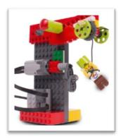
**Lego ® WeDo Construction Set** activities are all about adventure this session! The "Bungee Jumper" is wound up and and waits for activation. This happens when the motion sensor is triggered. The motor starts to turn the worm and cam gears, which trigger the slinging of the bungee jumper who is then stopped using a ratchet and pawl. This ceases the action lowering the jumper. If we didn't stop the jumper from falling he might hit the floor!
