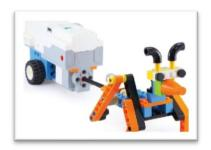
Once students get the hang of programming we will offer some simple builds like the Doggy Cart. This activity is driven by the motor turning the connected axle. This axle will turn the gears in the housing that contains the worm and 24 tooth gears that make the puppy's legs move. At first, the app will show the kids how to program specific moves, but as they build the bots, students can use what they have learned and program on their own. We are so excited to get building and
