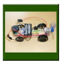
The students will make their own car that responds to its environment through a bumper switch. They will create the circuit and test the car with three different modes of transportation.
