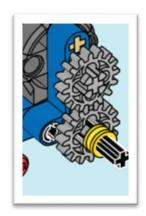
With a 1:1 gear ratio, speed can be increased using larger tires. Bigger tires have more friction with floor contact. By changing gear size, using a smaller gear on the motor and a larger gear on the axle we can greatly increase speed.
