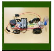
The students will make their own car that responds to its environment through a bumper switch. They will create the circuit and test the car with three different modes of transportation.
